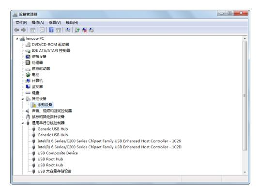
Right-click "unknown device", select "update driver software", manually add the driver of the device. Select the driver for installation from directory as showed in diagram below.
