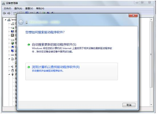
Select directory and install (driver located in the directory of CD directory [hardware drivers]). Select directory and install "CANalyst-II or USBCAN" (Depending on the model) in the directory of [hardware drivers]. Use the "Browse for Folder" window selects where the driver is:
