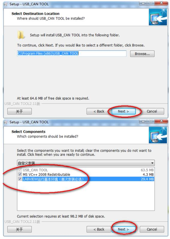
First time to install the USB-CAN please make sure to check "run Engine" .this installation package is needed for the application developed from the LABVIEW environment.
